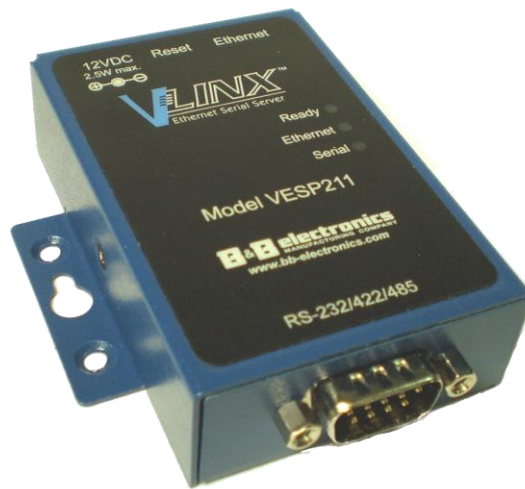
Figure 1. A VESP211 Serial Server
