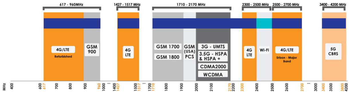
Indicates the LTE bands on which OMNI-0902 works  Indicates the WI-FI bands on which OMNI-0902 works
