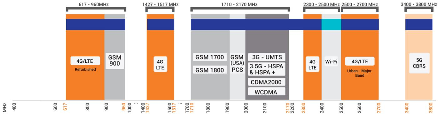
Indicates the 4G/5G bands on which OMNI-493 works   Indicates the WI-FI bands on which OMNI-493 works
